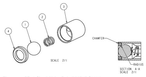
Figure 47: PR70 Check Valve Rebuild Kit (LC0093)
